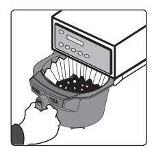
5 Slide the filled brew basket into the brew rails under the control panel. Slide it all the way back until it stops.
