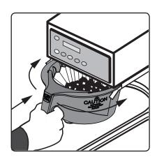
5 Slide the filled brew basket into the brew rails under the control panel. Slide it all the way back until it stops. Rotate the brew basket to direct the flow into the left or right tea container.
