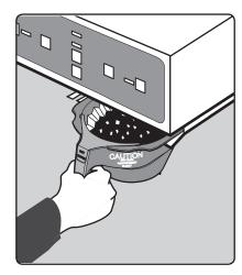
5 Slide the filled brew basket into the brew rails under the control panel. Slide it all the way back until it stops.
