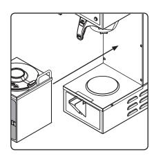
Place an empty satellite under the brew basket. Push it all the way back against the front cover. Press the WARMER button to preheat the satellite.
