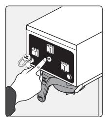
5 Determine the brew volume and flip the BREW SELECTOR switch to the desired size, position  $1 = \frac{1}{2}$ gallon, 2 = 1 gallon.
