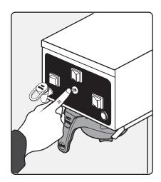
5 Determine the brew volume and flip the BREW SELECTOR switch to the desired size, position 1 = ½ gallon, 2 = 1 gallon.
