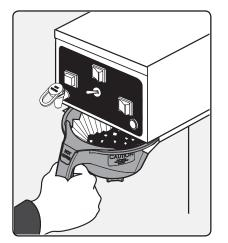
4 Slide the filled brew basket into the brew rails under the control panel. Slide it all the way back until it stops.
