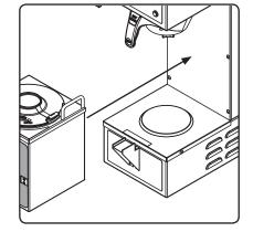
2 Place an empty satellite under the brew basket. Push it all the way back against the front cover. Press the WARMER button to preheat the satellite.
