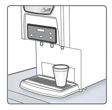
4 Place a cup under the spout for the desired flavor. If the dispenser is set for iced coffee, fill the cup with ice first.
