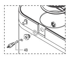
Water Level Probe Detail (Older Units)
