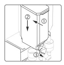
3 Reinstall each canister in the same spot it was removed from. Properly mate the gear socket on the back of each canister with the gear inside the dispenser. Turn the canister elbows downward and close the door.
