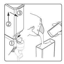
Open the front panel. On some models the panel swings to the right, on others, the panel swings up. Turn the elbow on each canister to be filled upward, then lift each canister up and out. Fill with powdered cappuccino product.
