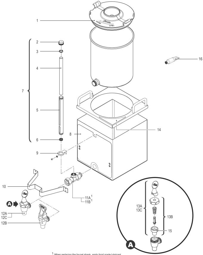
$^{1}$  When replacing the faucet shank, apply food grade lubricant (ITEM 16, not included) to both o-rings before installation.
