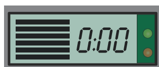
Level Gauge ON Digital Timer Readout ON LEDs OFF
