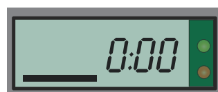
Level Gauge OFF Digital Timer Readout ON LEDs OFF
