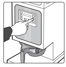
5 Make sure the grinder is on. On the grinder control panel, press the desired grind size/ brew volume button; SMALL, MEDIUM or LARGE. The grinder will start to grind coffee into the brew basket. Wait for the grinder motor to stop before removing the brew basket.
