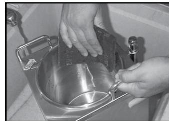
**NOTE -** Polish stainless steel surfaces with stainless steel polish after drying. This will prevent surface scratches and result in a cleaner appearance.
