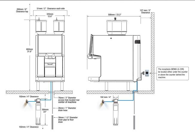
Notes: Access hole is only required if any of the utility hook-ups are located under the counter.
